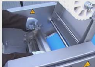
The quick and easy disassembly of the blade holders minimizes its changing times.
